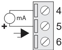
Connection to be used when the output loop must be powered directly by the Z109S-H module.
