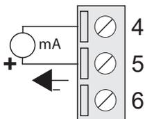
Connection to be used when the current loop power supply comes from the outside.
