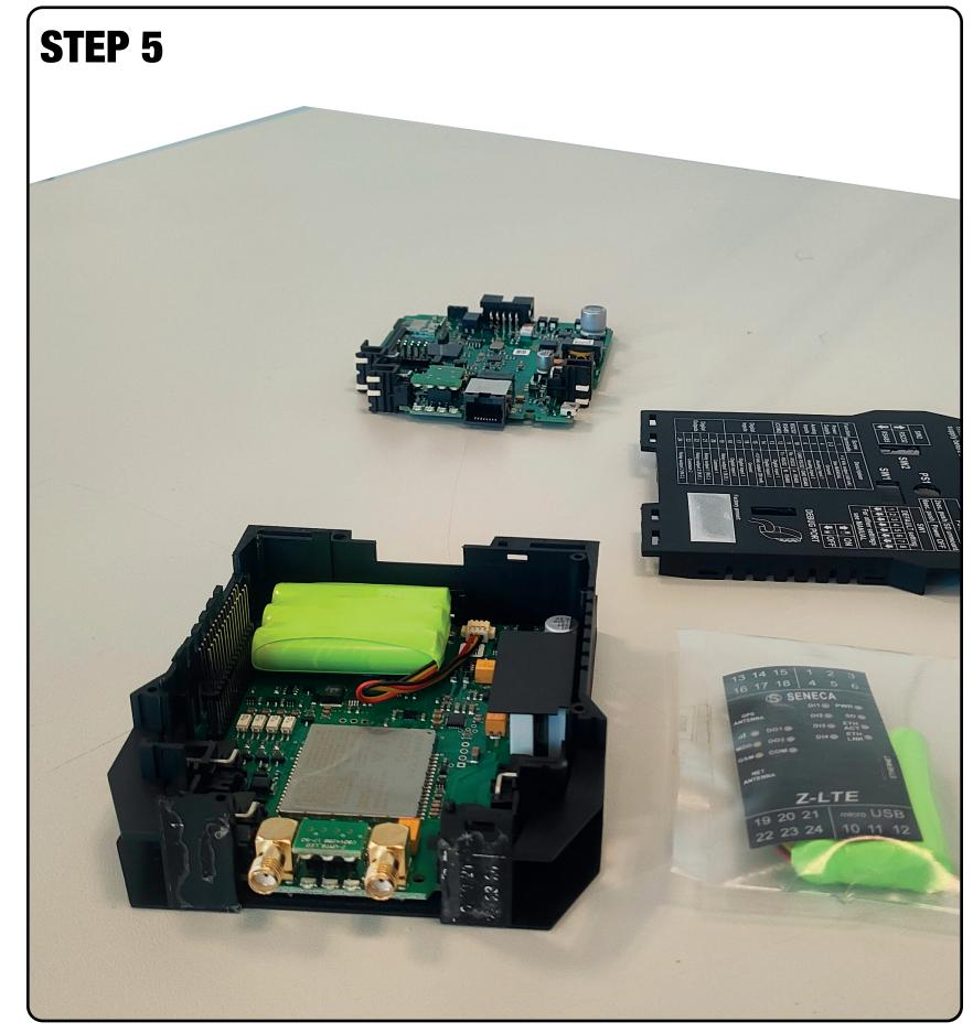
Disconnect the upper board to access the depleted and/or damaged battery pack.
