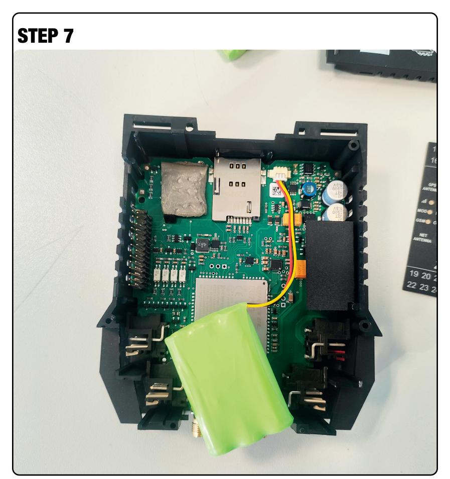
Connect the new battery to the contact pin.
