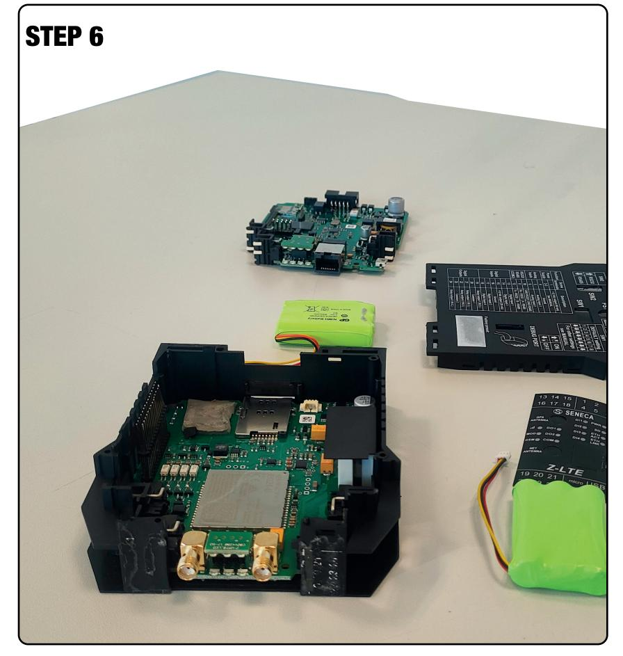
Disconnect the spent battery from the contact pin.
