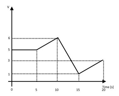
We then enter the coordinates of the points, the starting point of the ramp (time = 0) has the value of 5 V, we then enter point 1 with time = 0s, Value = 5V
