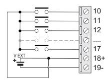
The digital inputs must be powered externally to function properly.(V EXT)
