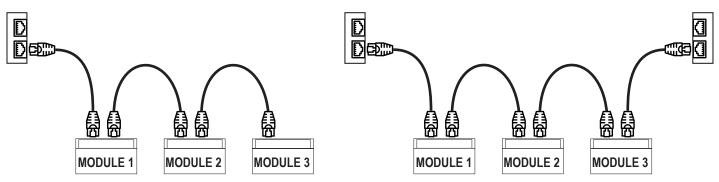
There must be no loops in the Ethernet cabling, otherwise the communication will not work. The modules and switches must be connected eliminating any loops. The following examples show the incorrect connections.
