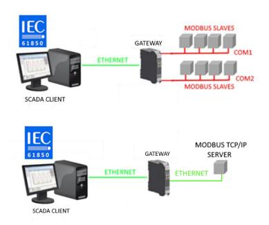
The Gateway, on the field side, works as a Modbus master / Modbus Client device and on the other side as an IEC 61850 server via Ethernet.
