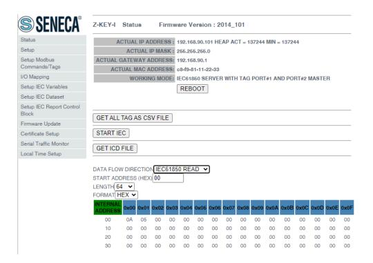
Now we press the "Start IEC" button, at this point the device restarts in IEC61850 mode (the webserver is now disabled), the operation could also be obtained by holding down the side button.
