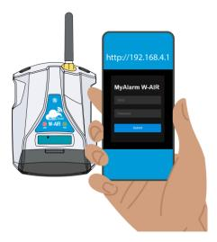
At this point the control unit will restart by connecting to the WIFI router, if the connection parameters have been entered correctly the "NET" LED is on steadily, flashing only when data is sent. Furthermore, the WIFI signal level appears on the main page:
