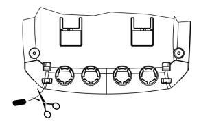
Once the pre-installed probe has been removed, connect the external NTC probe by wiring the cables to terminals 12 and 13 as shown in the figure below:
