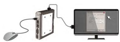
When cMT-FHDX is powered up and TV displays image, click the system setting button. (Default System Password: 111111) RJ-45 cable is necessary for connecting cMT-FHDX to your network.
