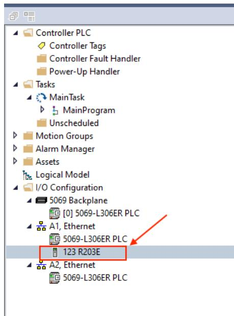
To simplify the acquisition of measurements and sending records to the device, you import the User Data Defined relating to R203-E:
