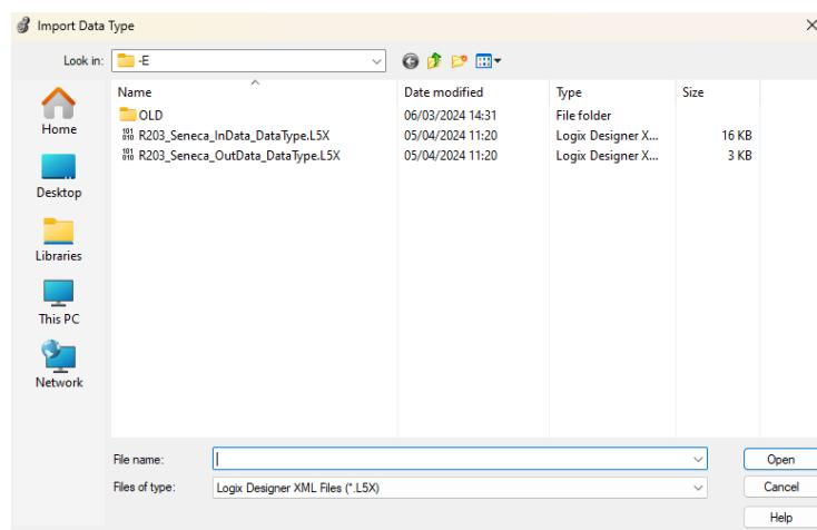
The InData will represent the measurements that come out of R203 towards the PLC, OutData are the tags that allow you to send commands to R203:
