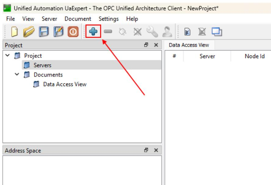
At this point under "Custom directory" we enter the IP address of the R203-U device (192.168.90.101 in the example) and the configured port (4840 in the example):
