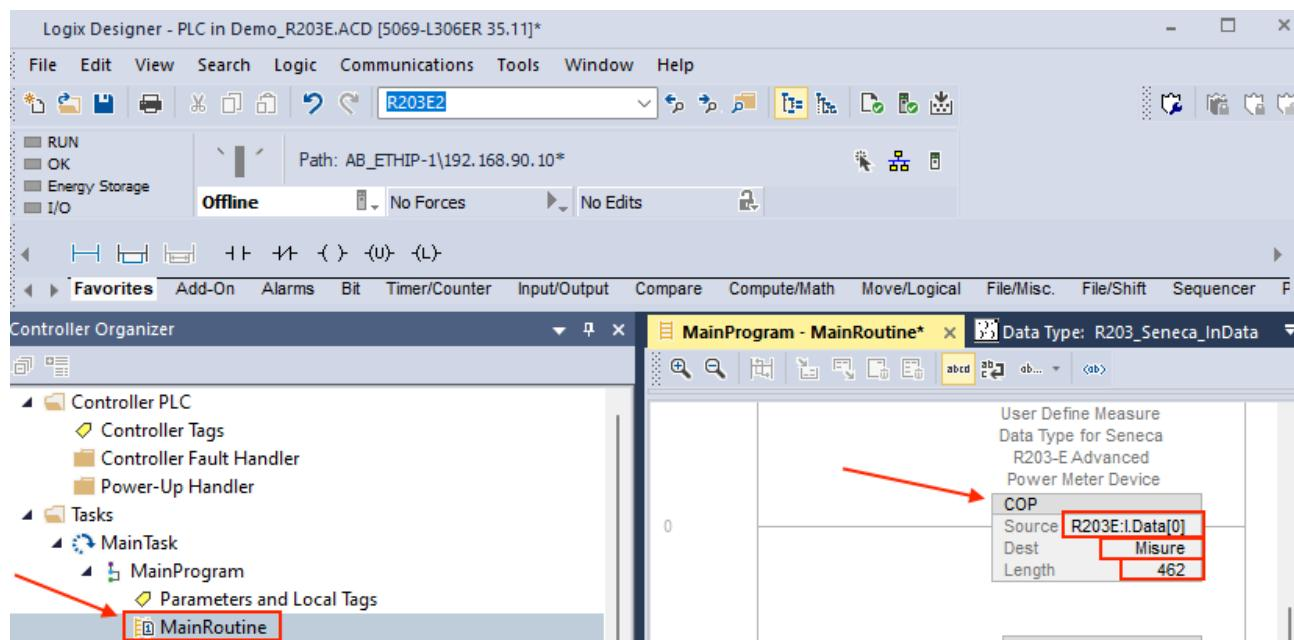
And then copy the values that you will control in the R203\_Seneca\_OutData structure into the data sent to the device:
