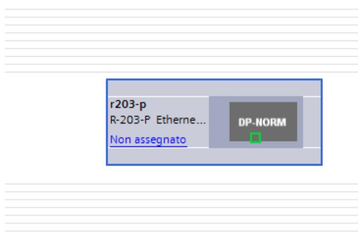
Now associate it to the PLC by clicking with the left mouse on "Not assigned" and then select the PLC:
