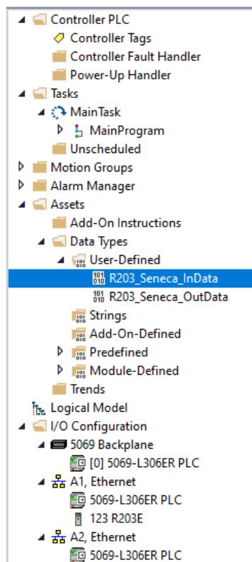
Now define the “Measurements” and “Outputs” with “R203\_Seneca\_InData” and “R203\_Seneca\_OutData” data type respectively:
