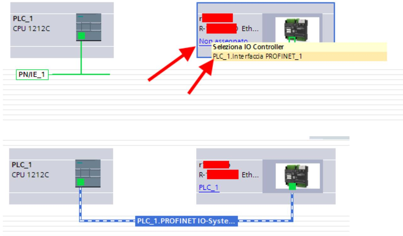
Click twice on the Seneca device and configure the IP address here too (for example 192.168.90.48):
