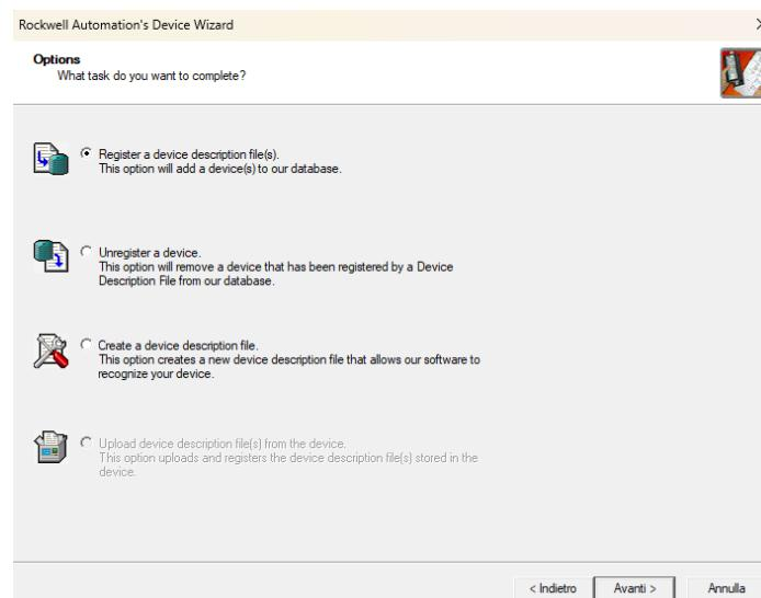
Select to register a single device and select the "R203-P.eds" file
