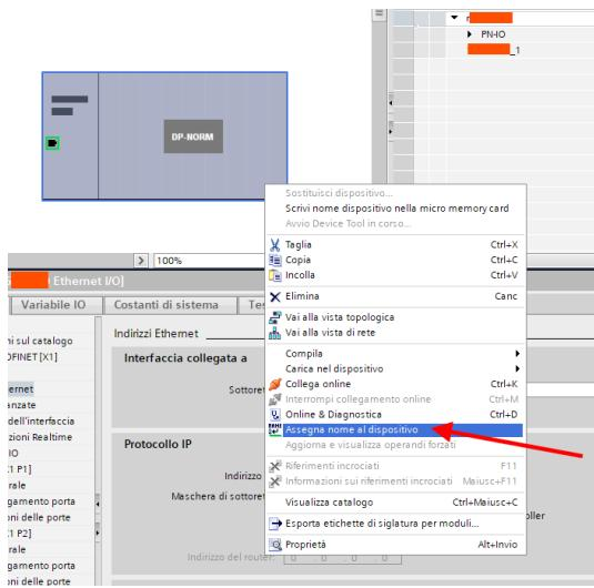
Scan the network with "Update list" and set (if necessary) the device name with "Assign name".
