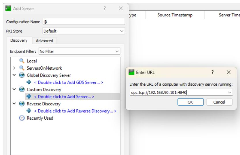
By pressing OK the server is added to the list, select the desired encryption:
