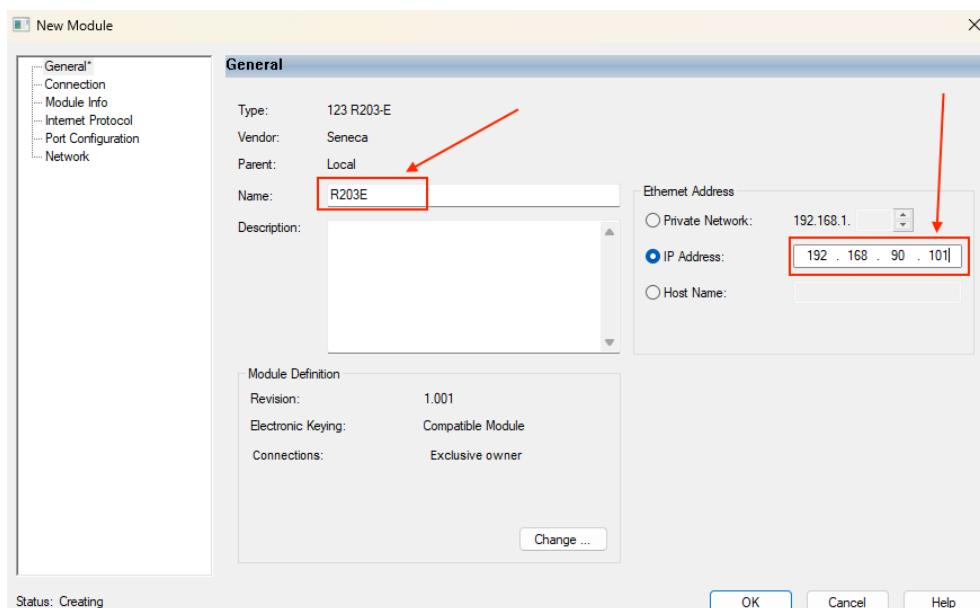
By confirming with OK the device is added:
