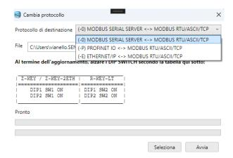
At the end of the operation, bring (only at the first power-on) the dip switches 1 and 2 to "ON" to force the device to default (see also the chapter "RESETTING THE DEVICE TO ITS FACTORY CONFIGURATION").
