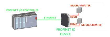
The gateway provides two different areas of 512 bytes for reading and 512 bytes for writing.
