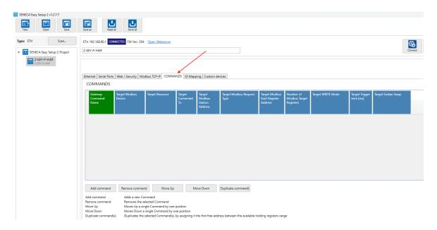
We add the reading of 10 coil registers relating to the 10 digital inputs of Z-10-D-IN:
