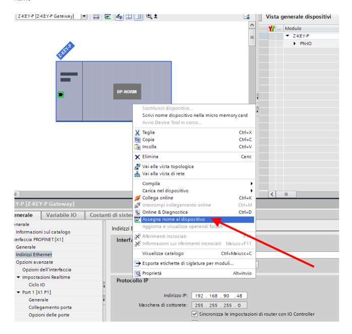
Scan the network with "Update list" and set (if necessary) the device name with "Assign name".
