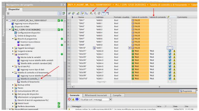
Here it is now possible to read inputs and force write outputs.
