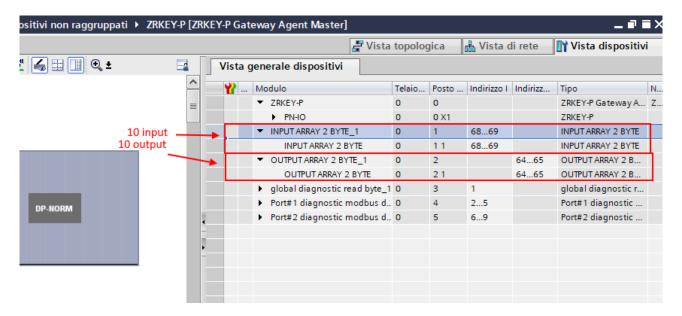
In particular, the 10 inputs are available at addresses I68 and I69 while the outputs are located at addresses Q64 and Q65.
