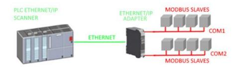
The Gateway, in the serial part, works as a Modbus master device and in the Ethernet part as a Ethernet /IP Adapter.
