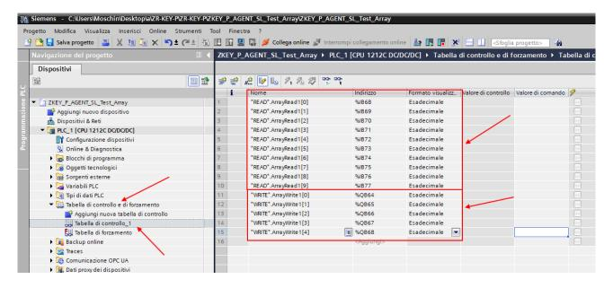
The 5 bytes of Profinet writing are the 5 bytes of reading from modbus (3 Modbus Bytes = 6 bytes). The 10 bytes of Profinet readings are the 10 bytes of modbus writing (5 Modbus registers = 10 bytes).
