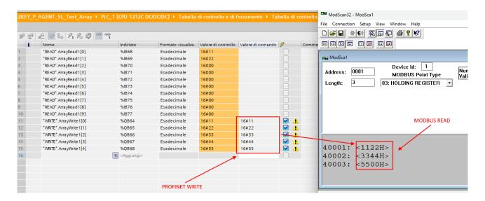
Writes from modbus are read by profinet like this:
