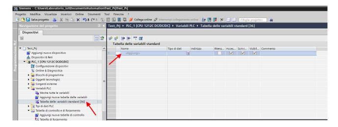
Add the tags related to the IO (in the example it is an R-16DI-8DO that is 16 digital inputs and 8 digital outputs). The addresses are written here:
