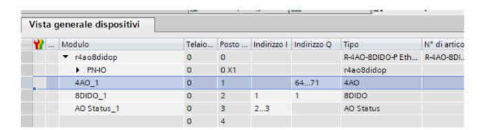
Bytes from Q64 to Q71 show the values of the 4 analog outputs in signed integer (2 bytes per output). byte I1 contains the 8 digital inputs (those configured as inputs), byte Q1 the 8 outputs (those configured as outputs).
