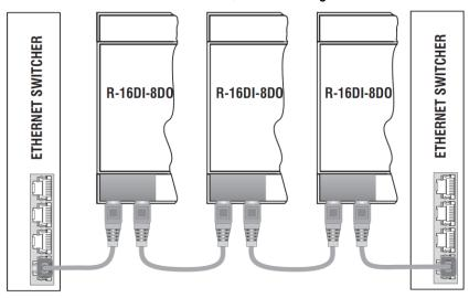
In the Ethernet wiring there must be no loop, otherwise the communication will not work, some examples of incorrect wiring are the following:
