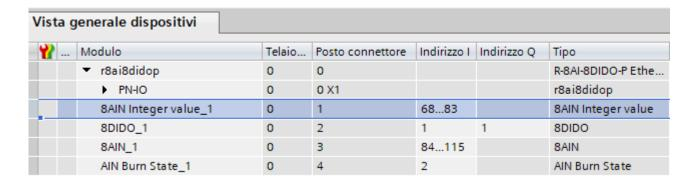
So byte I1 contains the 8 digital inputs (those as inputs), byte Q1 the 8 outputs (those configured as outputs). Bytes from I68 to I83 show the values of the 8 analog inputs (2 bytes per input).
