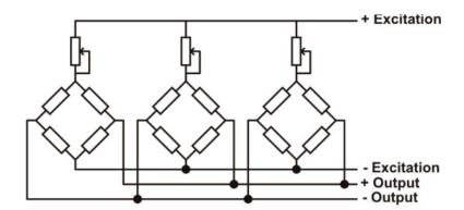
A variable resistor, independent of the temperature, or a typically 20  $\Omega$  potentiometer is inserted in the +Excitation cable of each load cell. There are two ways to trim the load cells. The first method is to adjust the potentiometers by trial, shifting the calibration weights from one corner to another.
