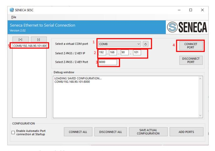
Please note that Seneca SESC can connect more than one serial device at the same time by adding another port with the "ADD PORTS" button. Each new port needs another gateway, so 2 different gateways are required to connect two serial devices to the same PC.
