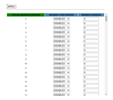
The first Column "Virtual Modbus Address" contains the virtual station address of master request.
