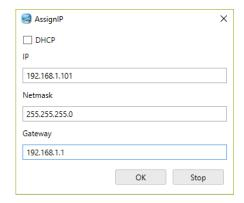
Confirm with OK. Now the device can be reached via Ethernet from your PC.
