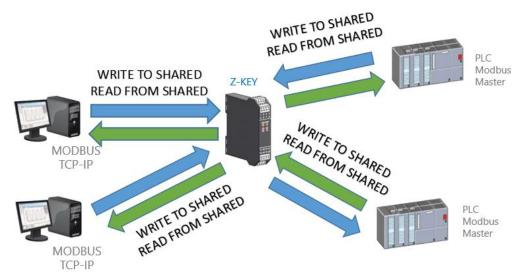
The shared memory of the gateway can be freely read and written by the Ethernet and/or by the serial ports.
