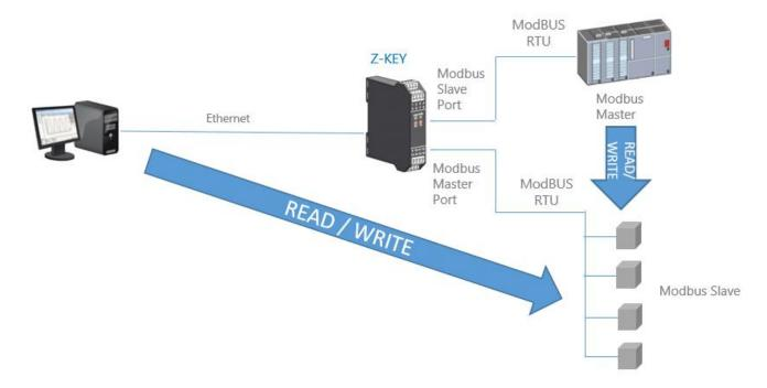
This function is possible because the Seneca Gateway uses an internal memory shared between the serial ports and the Ethernet port, where the data acquired from the serial Modbus Slave network are saved.
