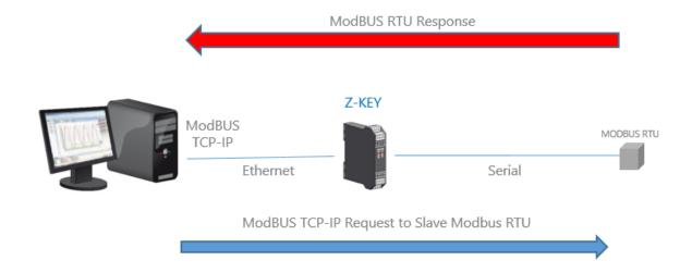
The Modbus TCP Client requests the reading/writing of a Modbus register via Ethernet, the gateway converts the request towards the serial slaves in Modbus RTU/ASCII and the Modbus RTU/ASCII response of the interrogated slave is subsequently converted towards the Modbus TCP Client.
