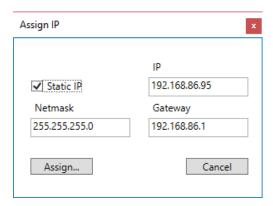
The software works on layer 2 level and it is therefore not necessary to have an Ethernet configuration compatible with the device you are looking for.
