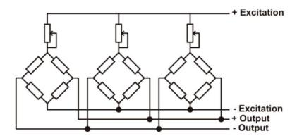
A variable resistor, independent of the temperature, or a typically 20  $\Omega$  potentiometer is inserted in the +Excitation cable of each load cell. There are two ways to trim the load cells. The first method is to adjust the potentiometers by trial, shifting the calibration weights from one corner to another. All the potentiometers must be adjusted so as to set the maximum sensitivity for each cell, turning them all completely clockwise. Then, once
