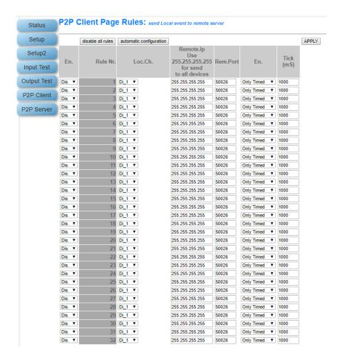
The "Automatic configuration" button allows you to prepare the rules for sending all the inputs available in the device in use.
