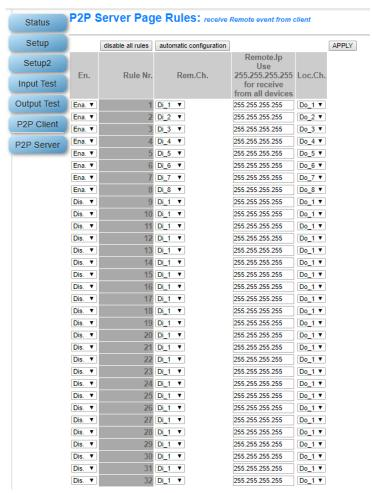
The "Automatic configuration" button allows you to prepare the rules to receive all the inputs on the outputs of the device in use.
