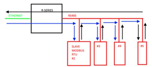
Each Modbus TCP-IP request with station address other than that of the R series device is converted into a serial packet on the RS485 and, in the case of a reply, it is turned over to TCP-IP.
