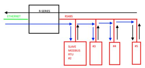
Each Modbus TCP-IP request with station address other than that of the R series device is converted into a serial packet on the RS485 and, in the case of a reply, it is turned over to TCP-IP.
