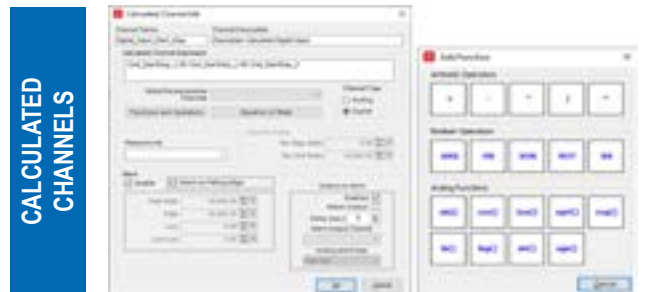
CALCULATED CHANNELS In addition to physical channels, the software allows the creation of calculated channels from a combination of imported channels and mathematical operators, with the possibility of applying different scaling for each channel.
