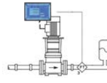
Pump regulation scheme based on flow measurement
