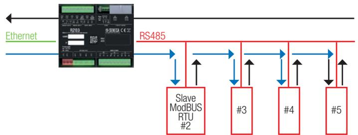
CONNESSIONE FAULT BYPASS
