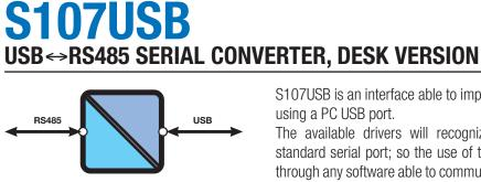
S107USB is an interface able to implement a RS485 serial port by using a PC USB port.
