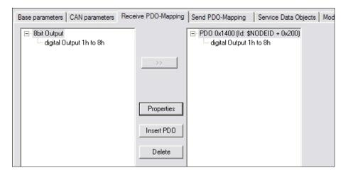
In the Receive PDO Mapping window, you can configure and view the PDO telegrams sent from the master to the slave. On the left you can see the data that the slave is able to receive through PDOs. In the figure case is an 8 digital outputs. On the right you see the link between the PDO and data output.
