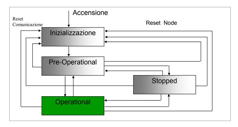
When the device is in PRE-OPERATIONAL state, communication via SDO is initiated. In this state, you can run the following settings via SDO:
