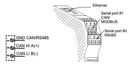
The pins CANH, CANL and GNDCAN are used for CANopen bus signals, the GNDCAN signal must be connected to obtain a robust communication. If it is necessary to use a T connection from the main bus line, see the following table for their maximum length (from ISO / DIS 11898):
