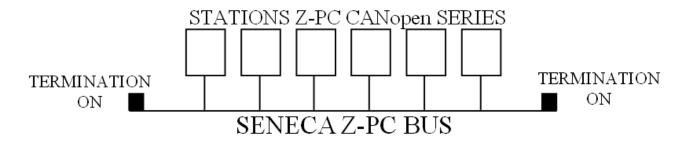
Note that a termination may be enabled directly to the TWS3/TWS64 stations through JP1 jumper.
