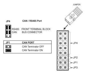
The connection is done by inserting the station back connector to the SENECA bus.
