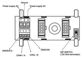
The connection to the bus of CANopen Slave station is done by inserting the back IDC10 plug in the bus Seneca.
