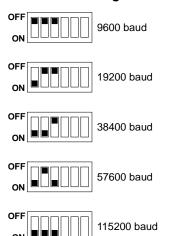
The dip switches used to select the speed and mode of the converter are situated next to the RS232 connection cable
