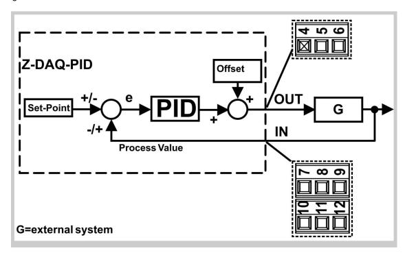
In particular, "e" means the difference between set-point and process-value:
