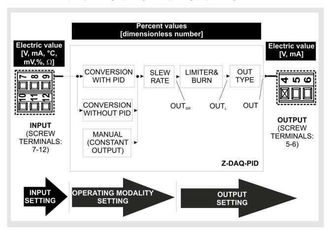
In particular, there are three operating modes, each of them allows to supply a ON/OFF output or an analog output:
