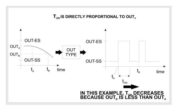
It is possible to limit upper time of high-state ON/OFF output (reg.40029) and to limit lower time of low-state ON/OFF output (reg.40030). The cycle time is reg.40028 (constant frequency of ON/OFF output=1/cycle time).
