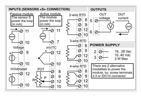
For potentiometer input connection: you must add externally a R=330  $\Omega$ , P=1 k $\Omega$ -100 k $\Omega$ .
